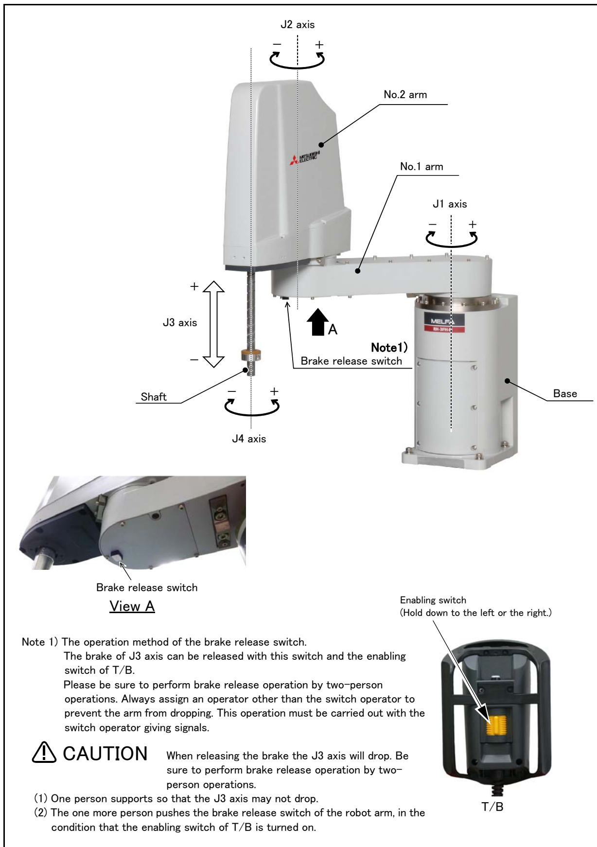
Fig.2-9 : Names of each part of the robot
